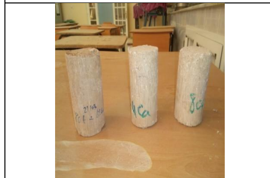
Figure 5: Tuff blocks reinforced with cardboard
