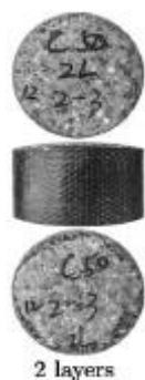
Figure 7. Tested concrete specimen wrapped by two layers of carbon fiber reinforced polymer [15].
